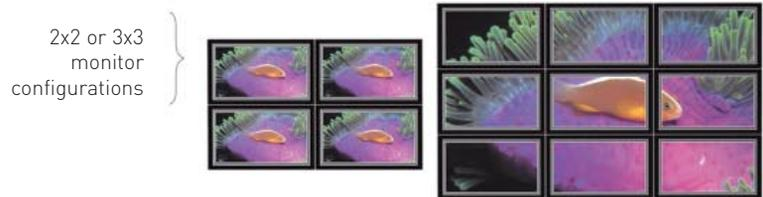
Built in **image matrixing** is possible in two configurations resulting in a 2x2 or 3x3 video wall. Internal processing allows the video to be split into quadrants eliminating the need for external matrix equipment.
